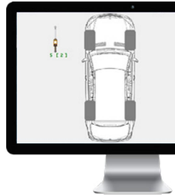
The **3D coordinates** of the tool are used by **ATC** or **VPG+** software to locate the tool and guide the operator in the correct assembly operation.
