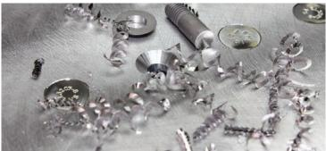
REDUCE FOD - 4 Fasteners removed with the E-Drill vs 1 fastener with a Twist Drill
